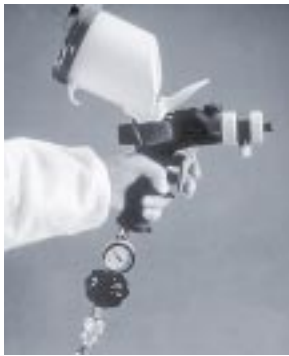
Well-balanced tool (sprayer) with a swivel connector for hoses
