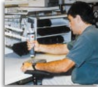
▲ In-line tool used on a horizontal surface makes the wrist and arm more comfortable
