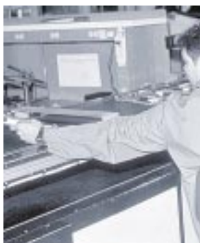
Work too far away— extended reach
