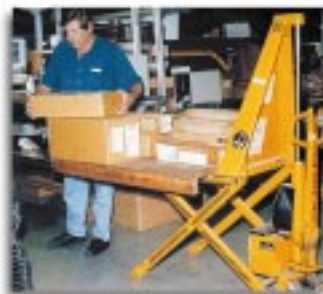
▲ Scissors lift provides a portable, height-adjustable workstation
