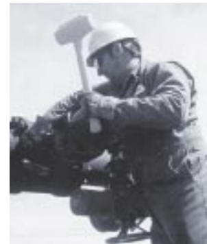
A dead-blow type hammer (composed of a nylon or plastic covering filled with metal shot)—reduces impact and contact stress from metal-on-metal hammering
