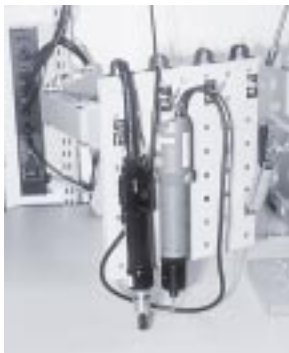
Triggerless tools—contact switches replace triggers
